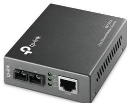
**TP-LINK CONVERTIDOR DE MEDIOS MC110CS 20.000 METROS 1 PUERTO FIBRA MONOMODO 1X RJ-45**
